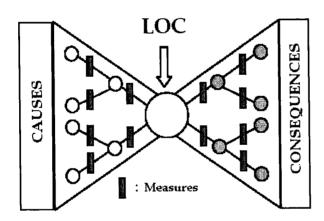
The centre of the diagram is the loss of containment event i.e. the "top event". The bow-tie left depicts the overall possible causes, which could lead to the
