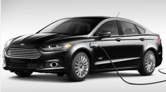
Ford Fusion Energi (PHEV) (2.0L I4 Benzinli + 7.6kWh Li-ion)
