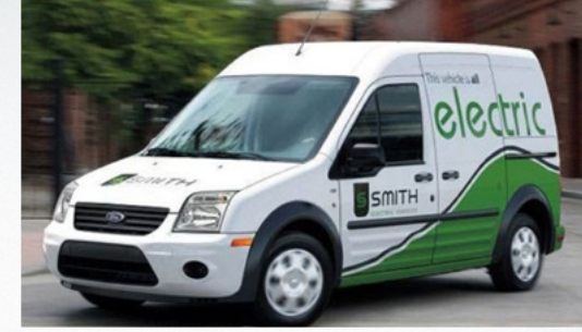
Transit Connect Electric (28kWh Li-ion)
