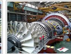
Blade Ring Assembly & Bolt Tightening
