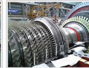
Blade Ring Assembly & Clearance Check
