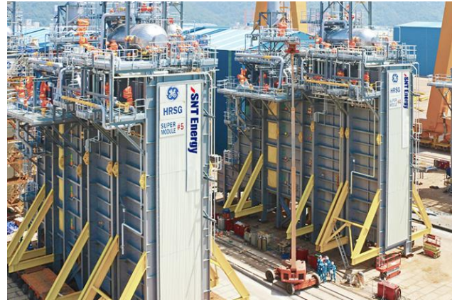
Heat Recovery Steam Generator
